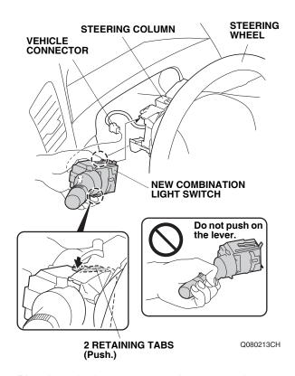
62. Plug the vehicle connector to the new combination light switch.
