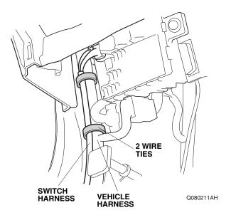
59. Unplug the vehicle connector from the combination light switch.
