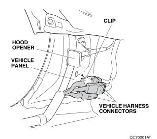
44. Remove the vehicle harness connectors from the vehicle harness 14-pin connector.Without another accessory connector
