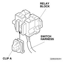
52. Install the relay to the switch harness relay block.
