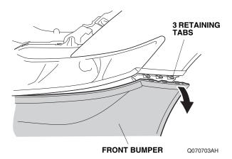
On each side, release five retaining tabs.
